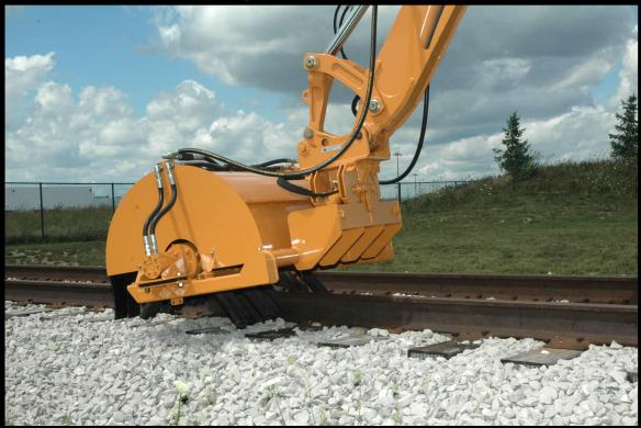
Mitchell Ballast Regulator Attachments for Backhoe Loaders and Hydraulic Excavators are used to regulate the ballast on railroad ties and track shoulders. The ballast elements are durable hard rubber elements that are the same elements used in product ballast regulators that are easily replaceable.
